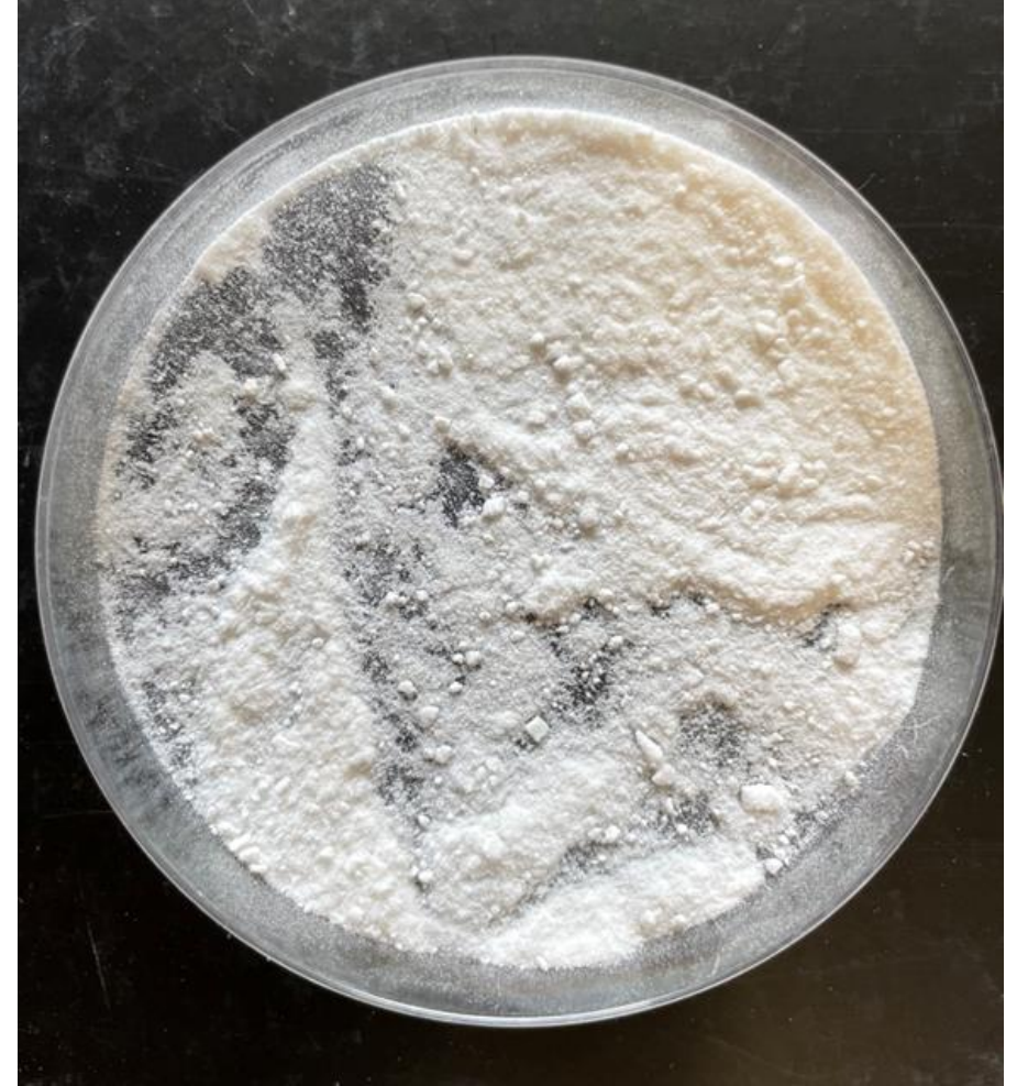
Lithium Carbonate produced from surface samples using Ekosolve™ Process
